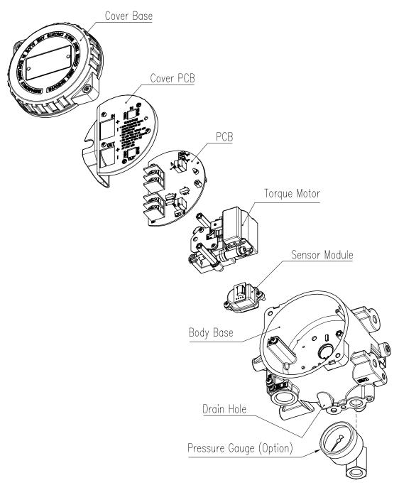
Fig. 2-1: exploded view
