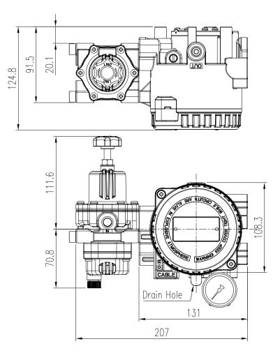
Fig. 2-3: YT-930 + Air filter regulator(YT-200) + Pressure gauge
