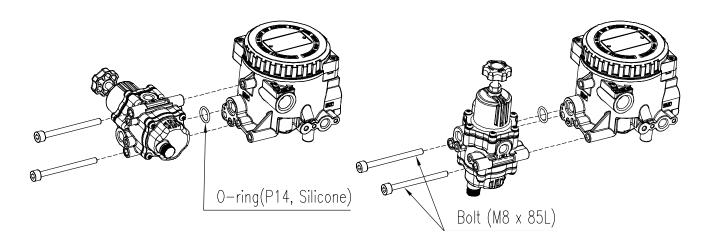
Fig. 2-3: Exploded view
