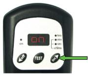
16. You can now press the left 'off/arrow down' button for decreasing the time or the right 'on/arrow up' button to increase the time.
