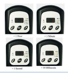
15. To change the ON time, simply press the right 'on/arrow up' button and 'on' will appear briefly on the display.
