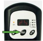
14. Time setting options; The ON and OFF time of the D-LUX timer can be programmed anywhere between 10ms and 99h.
